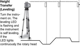
starts and the laser beam will be turned on. Attach the PLS HLD 1000 Detector at this reference point on a rod and move this height to zero. Now the respective difference in levels to the reference height can be measured on the ground. It is useful to use a flexible rod to measure positive and negative values simply.
