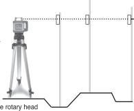
continuously the rotary head starts and the laser beam will be turned on. Attach the PLS HVD 505 Detector at this reference point on a rod and move this height to zero. Now the respective difference in levels to the reference height can be measured on the ground. It is useful to use a flexible rod to measure positive and negative values simply.
