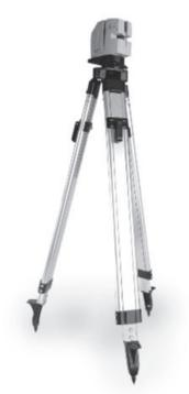
When using your PLS laser on a tripod secure the top component of the adapter to the tripod stud. Secure the PLS laser to the adapter and position the down point of the laser to point through the tripod handle, or cantilever the tool so the down point can be seen between the tripod legs. You can now adjust the laser for square layout using the down point as your spring point and capturing the square laser lines with your PLS SLD Detector.
